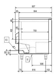
Drain Electrical inlet (power) ΕI Refrigerant Outlet
